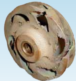
Above: cavitated impeller from commercial pool pump
